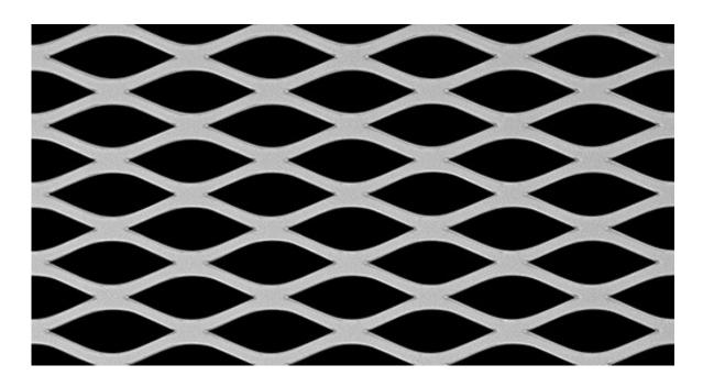
LW Aperture:32.77mmStrand Width:3.18mmSW Aperture:10.92mmThickness:1.50mmWeight:4.41 kg / m2Open Area:63%
